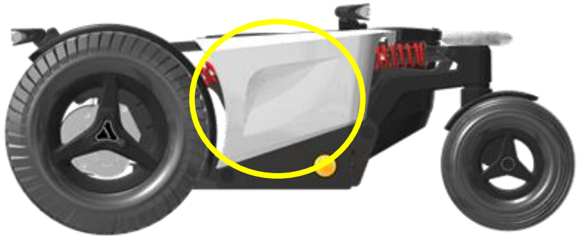
The battery box
