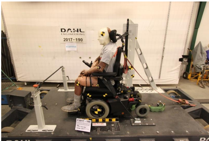
Evo Lectus crash test using Dahl Docking station.
