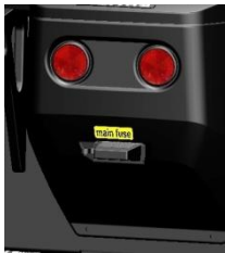
Position of the main fuse
