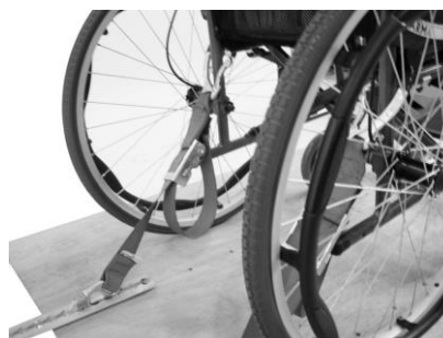
Fitting the rear restraint
