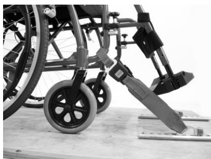
Fitting the front restraint
