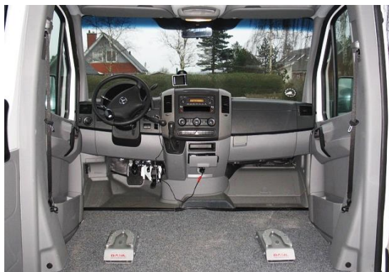
Dahl docking station mounted on the floor
