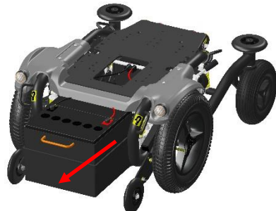
pulling out the battery box
