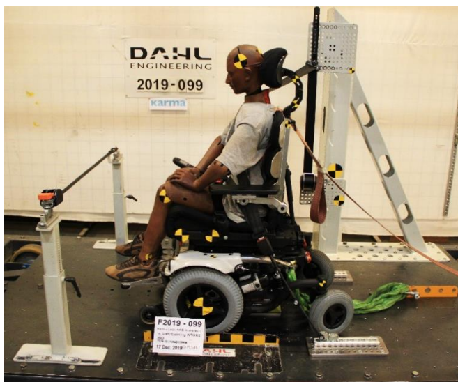
Leon F Kameleon crash test using Dahl Docking station
