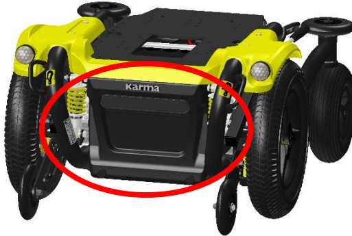
The front and rear battery box
