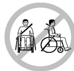
Incorrect seat belt position
