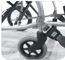
Fitting the front restraint
