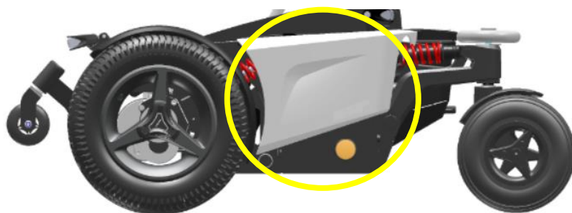
The battery box
