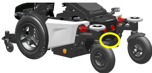
position main fuse
