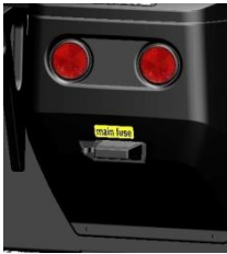
position of the main fuse
