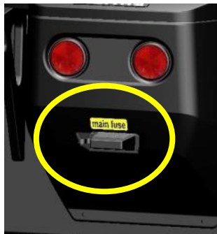
place of the main fuse
