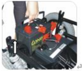
11. Lift up the battery by its handle.
