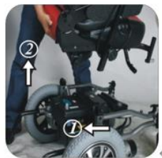
5. Lift and pull the seat backward to remove it from the base frame.↵
