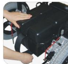
6. Unfasten the Velcro from the bottom of the battery box.↵
