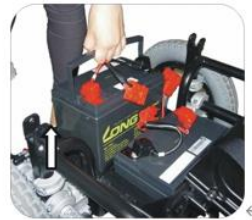
9. Lift up the battery by its handle.
