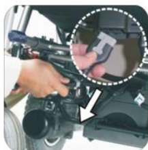
1. Disconnect controller wire.↵
