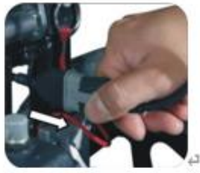
5. Remove the cable from the transmission connector.
