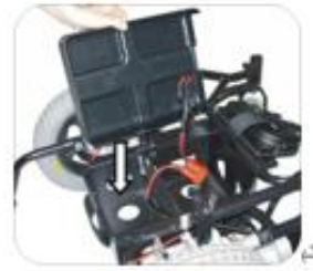
12. After removing the batteries, close the battery box cover.
