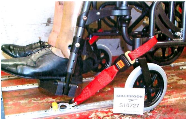
Fitting the front restraint
