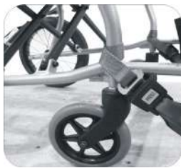
Fitting the front restraint
