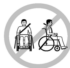
Incorrect seat belt position
