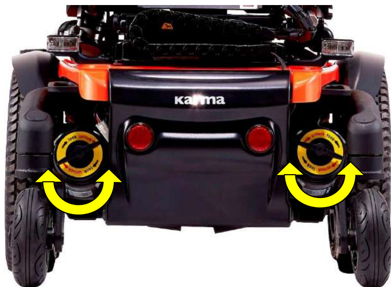
Testing the brake release
