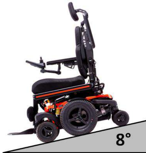
Max. acceptable downhill slope
