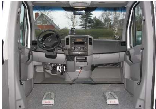
Dahl docking station mounted on the floor
