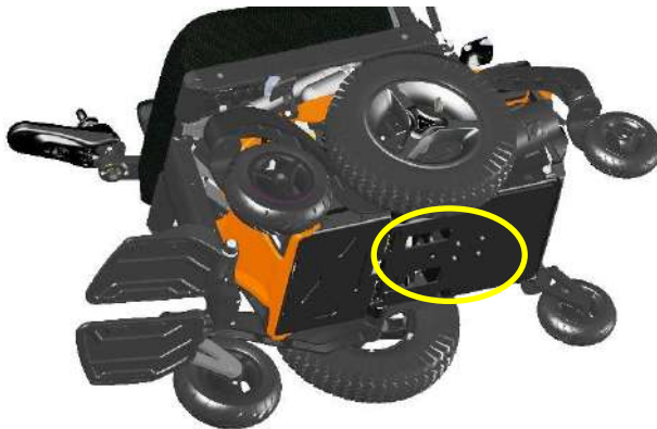
Dedicated holes for mounting Dahl lock plate
