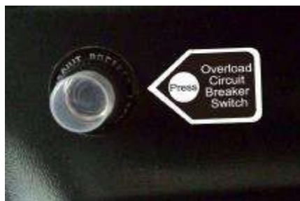
Push button of the circuit breaker
