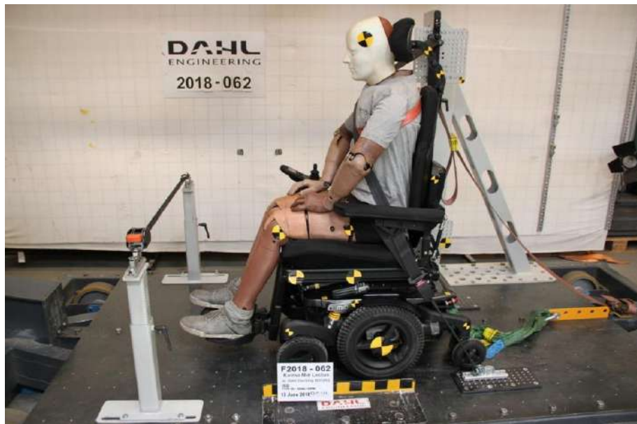
Mid Lectus crash test using Dahl docking station
