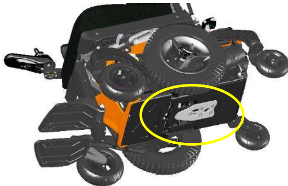
MID chassis with Dahl Docking plate mounted.
