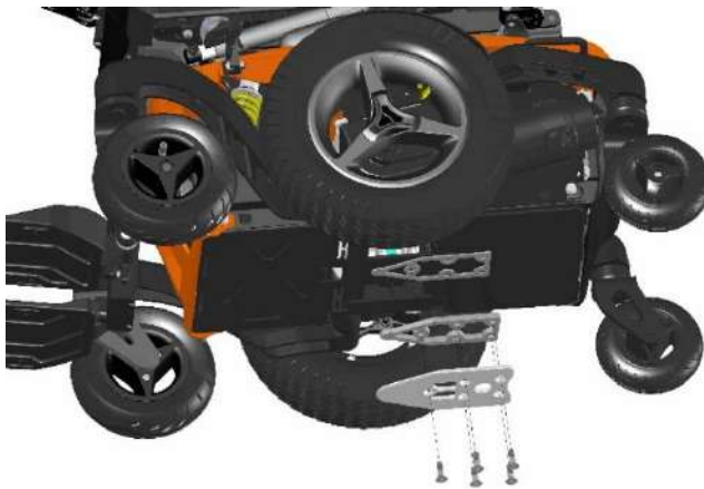
Mounting the Dahl lock plate on to the MID chassis
